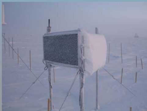
Static snow buildup on leeward panel
