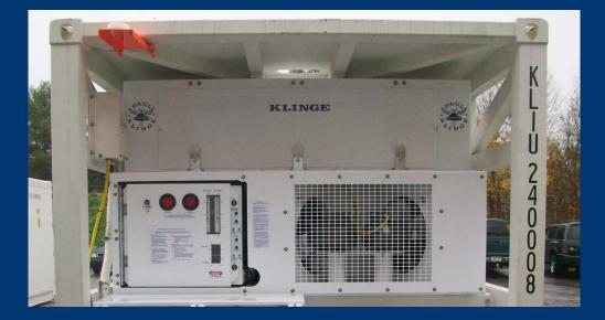
» Each reefer unit is capable of maintaining the required cargo bay temperature as low as -30°C (-22°F) automatically, using cooling and defrost cycles during operation.
