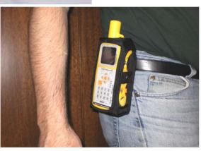
Nylon carry case with open front option – no plastic cover to shatter in the cold
