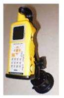
Direct Connect Kit provides filtered power from vehicle, RAM Mount Bracket for ATV/vehicle/snowmobile mounting
