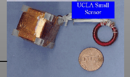
UCLA Magnetometer Sensor w/ integrated Thermistor
