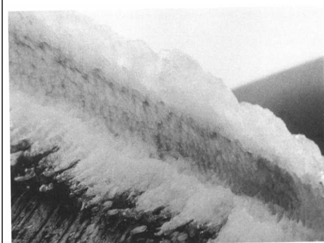
Figure 2-f Close-Up Of Ice Formation With Runback. Photo illustrates in-flight wing leading edge ice formation. NASA Photo.
