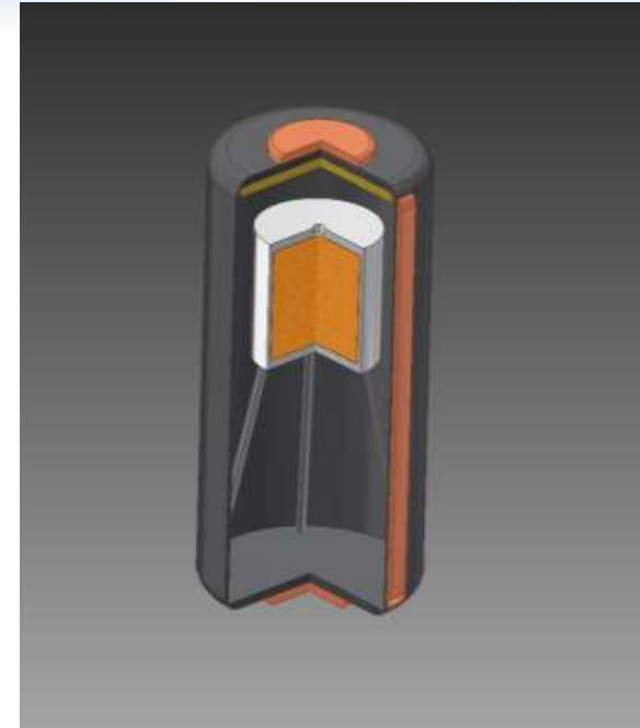
Estimated RPS source for 5 We– 400 g, “D cell” size
