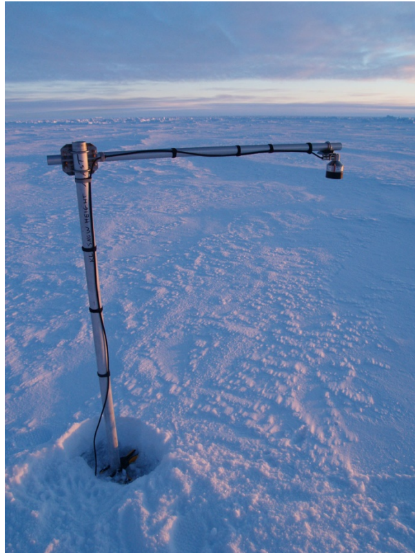
Snow Height Buoy (WHOI) snow height sensor, left to drift on floes
