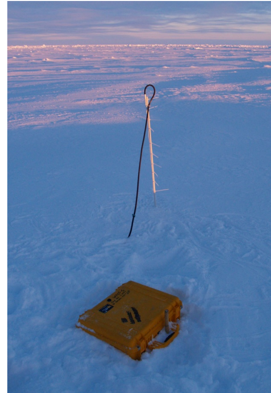
Ice Mass Balance Buoy (SAMS) thermistor string to measure snow and ice thickness, left to drift on ice floes
