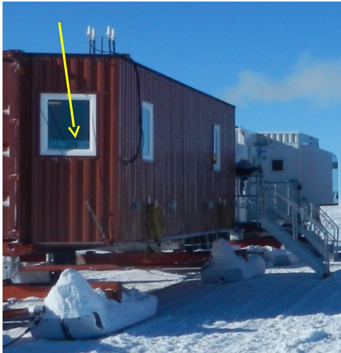
RUDICS based camera system mounted in window of kitchen sled
