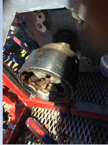
Broken spider gear due to engine/ compressor gearing mismatch
