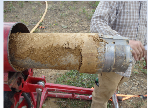
Clogging due to conditions and some drilling inexperience. Learning curve.
